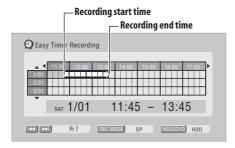
As you move the cursor around the grid, an arrow stretches from the start time to the current cursor position, representing the length of the recording. A recording of up to six hours can be set.
